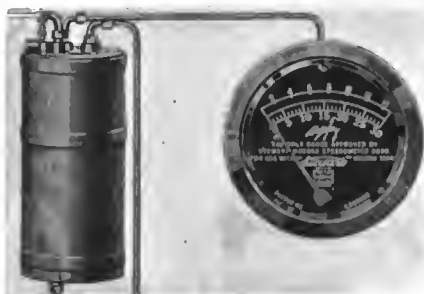
J-A-Y vacuum gage which is a complete index to the Stewart fuel feed system
